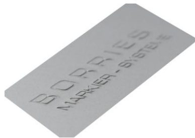
Test marking with 3 mm font height on eloxadized aluminum
